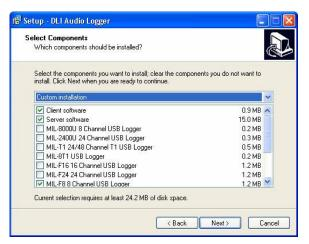
Next, select the components to install. Three components are critical: Server Software, Client Software, and the MIL-F8 USB Logger.
