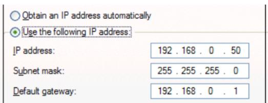
The screenshot shows the 'Internet Protocol Version 4 (TCP/IPv4) Properties' dialog box. The 'Use the following IP address' radio button is selected. The IP address is set to 192.168.0.50, the Subnet mask is 255.255.255.0, and the Default gateway is 192.168.0.1.
