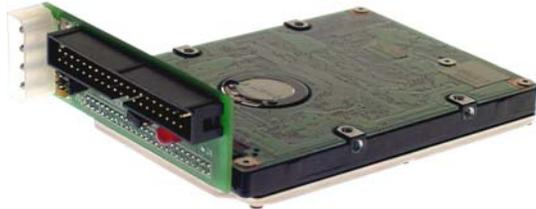
**Warning:** Some notebook drives are not “keyed”. Be extremely cautious when mating the adapter board to notebook drives. Incorrect orientation will cause damage to the notebook adapter, and possibly to the drive as well. The adapter card should project above the metal surface on the top of the drive, not below it. Both rows of connector pins must be completely inserted in the adapter.
