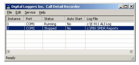
ANI, ALI, or SMDR data streams may be logged using our call detail recorder utility. This utility logs up to 8 RS-232 serial ports simultaneously.
