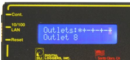
Outlet (port or relay) status shows on the first line. The outlet name or time/date of last modification shows on the second line. Three symbols are used for relay status + (ON), - (OFF), and \* (LOCKED). In this example, relay 1 is locked ON, the even numbered relays are ON, and relays 3.5.7 are OFF. The flashing cursor indicates outlet 8 is selected:
