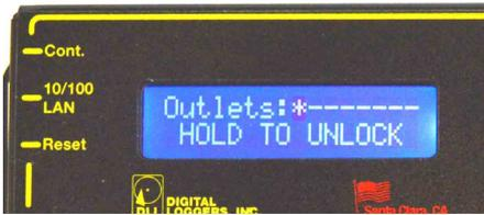
Press '0' and hold for a few seconds to unlock. Similarly, if the outlet is currently in the OFF state it can be locked by holding '0' and unlocked by holding '1'.
