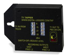
To set up combine mode, first select an input level. The default level of -20dBm will work fine in most installations. For -20, set switches 1,2, and 3 Off, and switch 4 On. On is to the right, Off is to the left when looking at the front of the T-1 Tapper.
