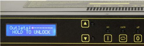
Press '0' and hold for a few seconds to unlock. Similarly, if the outlet is currently in the OFF state it can be locked by holding '0' and unlocked by holding '1'.
