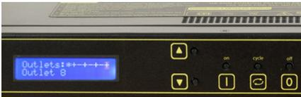
Press any key to activate the keypad. “Keypad Locked” will be displayed if keypad was locked by the admin on the setup page.
