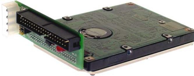
**Warning:** Notebook drives are not “keyed”. Be extremely cautious when mating the adapter board to notebook drives. Incorrect orientation will cause damage to the notebook adapter, and possibly to the drive as well. The adapter card should project above the metal surface on the top of the drive, not below it.
