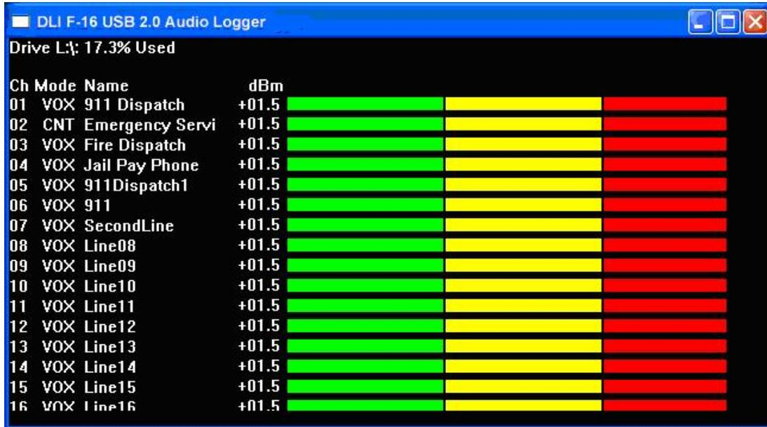
The recording mode for each line (for example VOX, LOOPSTART or OFF) is displayed to the left of the line name. The recording level for each line appears in color when that line is recording.
