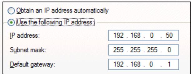
The image shows a screenshot of the Windows IP configuration dialog box. It has two radio buttons at the top: 'Obtain an IP address automatically' (which is unselected) and 'Use the following IP address:' (which is selected and highlighted with a dashed border). Below these are three input fields: 'IP address:' with the value '192 . 168 . 0 . 50', 'Subnet mask:' with the value '255 . 255 . 255 . 0', and 'Default gateway:' with the value '192 . 168 . 0 . 1'.
