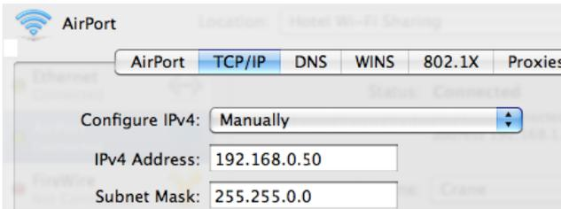
Make the changes shown. Point your browser at 192.168.0.100 and log in. Find detailed instructions at [digital-loggers.com/mac\\_ip\\_setup.pdf](http://digital-loggers.com/mac_ip_setup.pdf)
