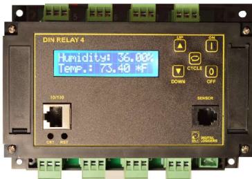
DIN Power relay with WiFi
