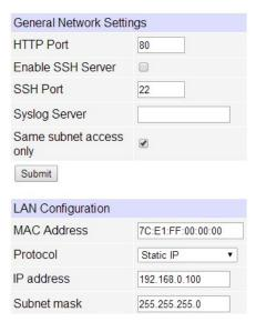
The IP address of the controller usually must match the "class C" of your system. In other words, the first three bytes (192.168.0) must match the IP on your computer to access the controller. Using a **Ping** utility is a good way to confirm a valid network configuration. An "unreachable" report from **Ping** indicates a misconfigured network.
