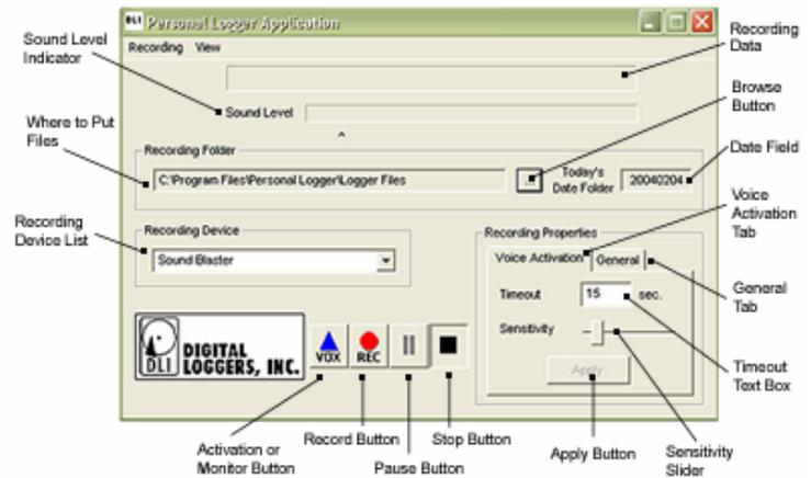
adjust both the MIC level slider in the Windows Audio Control Panel and the slider on the Personal Logger for best audio quality. If either level is set too high, touch-tones and caller-ID won't decode properly.
