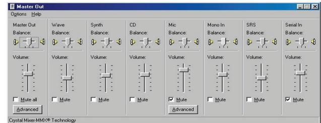
Slide the volume up on the MIC level, and uncheck MUTE. If your control panel has a SELECT box, select only the microphone, and de-select the others.
