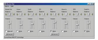
Slide the volume up on the MIC level, and uncheck MUTE. If your control panel has a SELECT box, select only the microphone, and de-select the others. Windows Audio Control Panel Shortcuts In XP, click Start then Run and enter sndvol32 -r In Vista or Windows 7, click Start then Run then mmsys.cpl ..1
