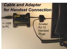
are provided. Use them to connect from the handset to the recording module. Connect the USB cable to any available USB port on your PC.
