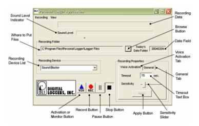
adjust both the MIC level slider in the Windows Audio Control Panel and the slider on the Personal Logger for best audio quality. If either level is set too high, touchtones and caller-ID won't decode properly.
