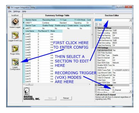
Six recording trigger (VOX) modes can be used to start and stop recordings.
