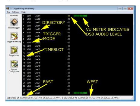
The main screen lists each DS0 timeslot in order. This example shows "combine" mode with 24 channels displayed.
