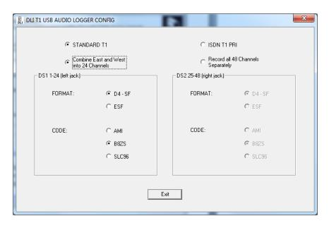
At this point, you should select the T-1 format and line code. Set FORMAT to D4 or ESF to match the T-1. Set CODE to match the T-1 line code. This is normally marked on the jack, or you can get this information from your installer. ISDN PRI is now the most common configuration.
