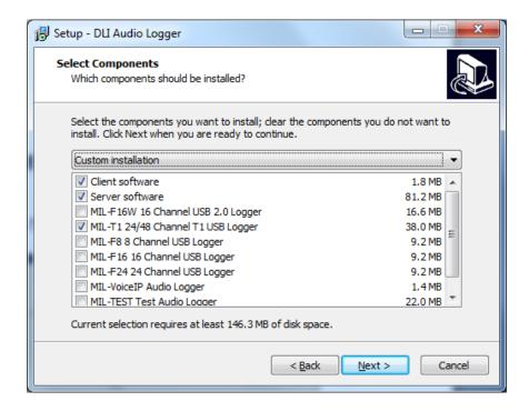
Select the components you wish to install. In a standard T-1 installation, these three components should be selected:
