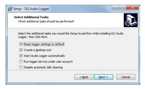
To starting recording automatically after login, check 'Start Audio Logger Automatically" If a machine is left unattended, this restores operation in the event of a power failure and subsequent reboot.
