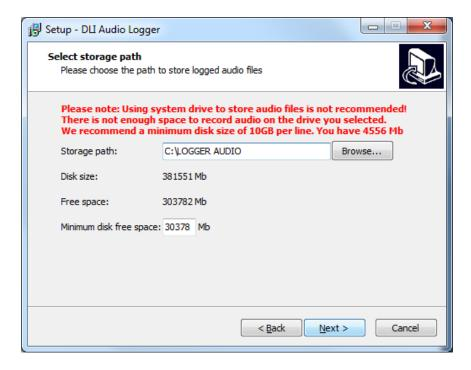
We highly recommend that a separate hard disk drive or SSD is used for call recording. By keeping the audio files on a separate disk drive, you are assured that other applications which use the system drive won't interfere with audio streaming. A 3-4TB hard drive typically works well.
