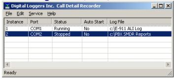
ANI, ALI, or SMDR data streams may be logged using our call detail recorder utility. This utility logs up to 8 RS-232 serial ports simultaneously. Download this utility from:
